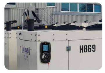
Diesel Generator NOx test
