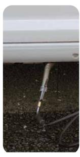
In cab heater CO<sub>2</sub> test with EP5 probe
