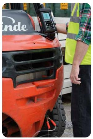
Fork lift truck emissions test
