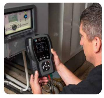
Testing boiler efficiency
